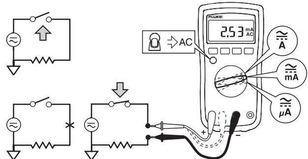
**Figure 2. Measuring AC and DC Current**
