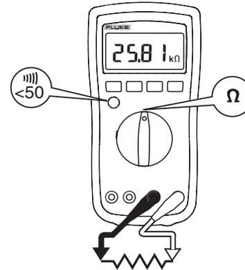
Figure 3. Measuring Resistance/Continuity
